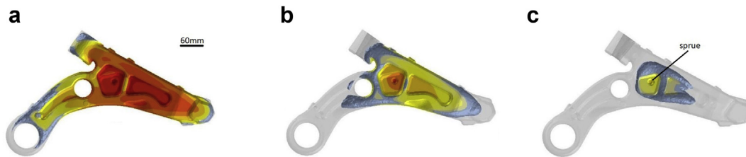
Fig. 15 – Solidification sequence - represented by contours of solid fraction limited to 0.7.
