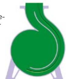
Figure 14. Casting design for a carbon steel pump casing.
