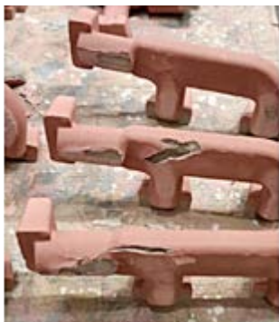
Fig. 8. Cracked cores after drying
