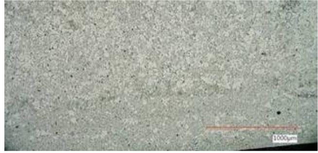
**Figure 14:** Aural™-2 microstructure after PSHT at 460 °C.
