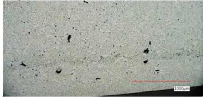
**Figure 15:** Aural™-3 microstructure after SHT at 500 °C.
