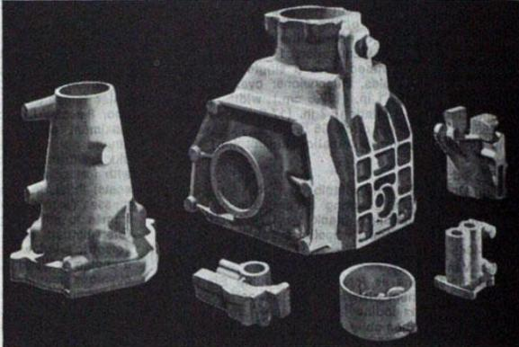
GRAVITY DIE CASTINGS produced for ROLLS-ROYCE LIMITED
